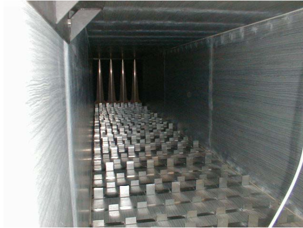
Fig. 2: Spires and roughness elements inside the Environmental wind tunnel of the IT.
